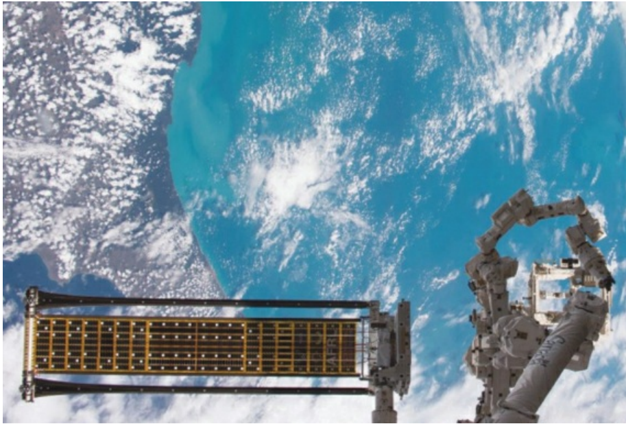
Our ROSA solar array was demonstrated on the International Space Station in 2017. Credit: NASA
